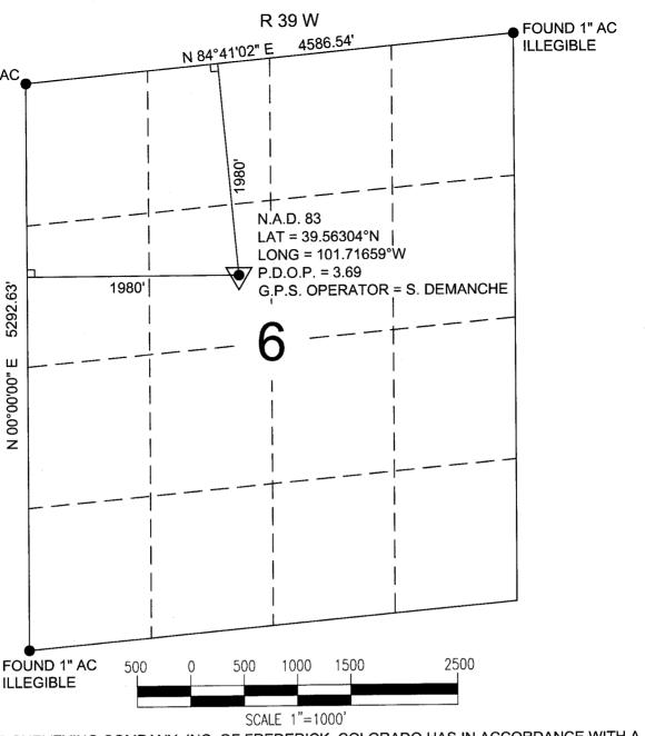
POWER SURVEYING COMPANY, INC. OF FREDERICK, COLORADO HAS IN ACCORDANCE WITH A NOBLE ENERGY INC. OF DAN CASPER **REQUEST FROM** LOCKARD 22-6 DETERMINED THE LOCATION OF OF SECTION 6 1980' FNL & 1980' FWL TO BE OF THE 6th PRINCIPAL MERIDIAN, 6 SOUTH \_\_\_, RANGE \_\_\_\_ 39 WEST TOWNSHIP KANSAS STATE OF SHERMAN COUNTY OF
