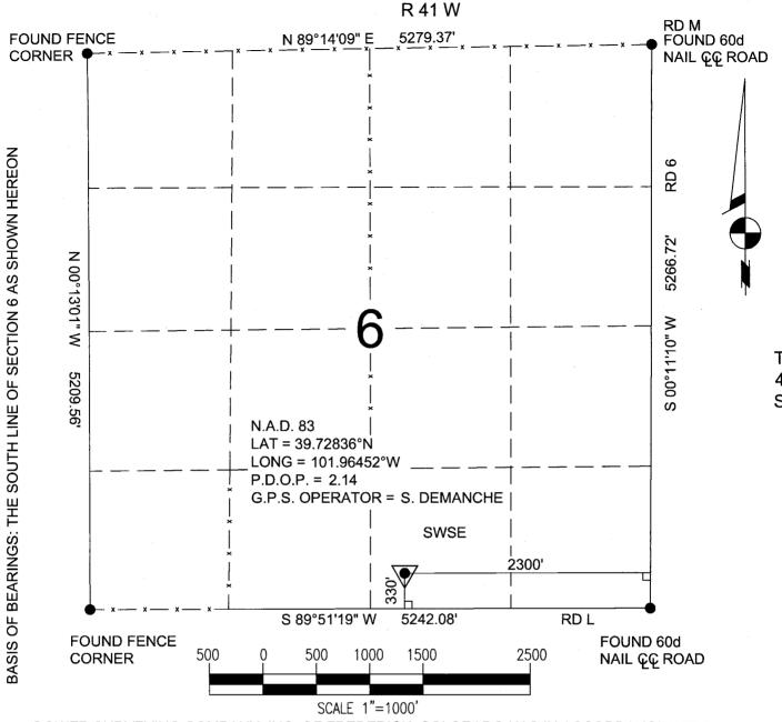
POWER SURVEYING COMPANY, INC. OF FREDERICK, COLORADO HAS IN ACCORDANCE WITH A REQUEST FROM DAN CASPER NOBLE ENERGY INC. DETERMINED THE LOCATION OF ZIMBELMAN 34-6 330' FSL & 2300' FEL OF SECTION TO BE TOWNSHIP 4 SOUTH , RANGE \_\_\_ OF THE 41 WEST 6th PRINCIPAL MERIDIAN. COUNTY OF STATE OF CHEYENNE **KANSAS**
