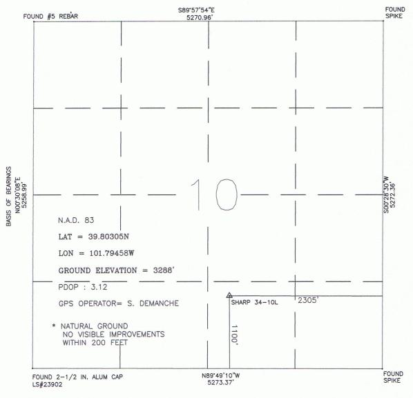
I HEREBY STATETO PETROLEUM DEVELOPMENT CORP THAT THIS WELL LOCATION CERTIFICATE INDICATES THE WELL SHARP 34-10L TO BE LOCATED 1100' FSL AND 2310' FWL, SEC 10, T4S, R42W, 6TH P.M. CHEYENNE COUNTY, STATE OF KANSAS
