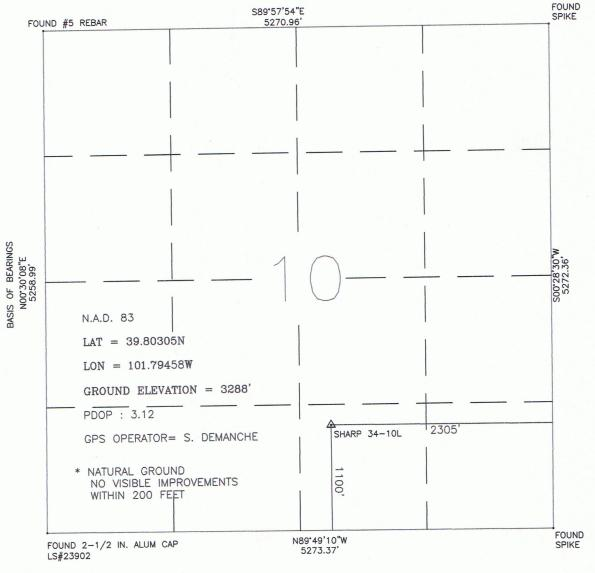
I HEREBY STATETO PETROLEUM DEVELOPMENT CORP THAT THIS WELL LOCATION CERTIFICATE INDICATES THE WELL SHARP 34-10L TO BE LOCATED 1100' FSL AND 2310' FWL, SEC 10, T4S, R40W, 6TH P.M. CHEYENNE COUNTY, STATE OF KANSAS
