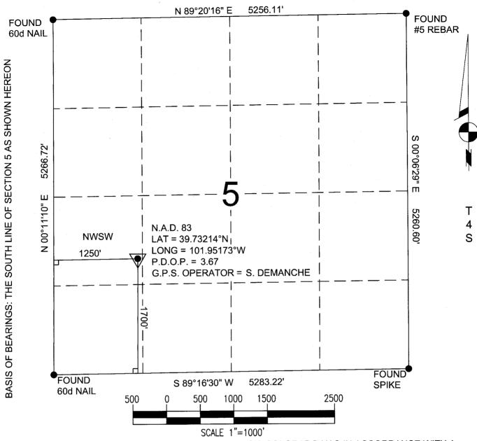
POWER SURVEYING COMPANY, INC. OF FREDERICK, COLORADO HAS IN ACCORDANCE WITH A NOBLE ENERGY INC. OF REQUEST FROM **DAN CASPER WIESE 13-5** DETERMINED THE LOCATION OF OF SECTION 5 1700' FSL & 1250' FWL TO BE TOWNSHIP 4 SOUTH , RANGE 41 WEST OF THE 6th PRINCIPAL MERIDIAN, STATE OF **KANSAS** CHEYENNE COUNTY OF
