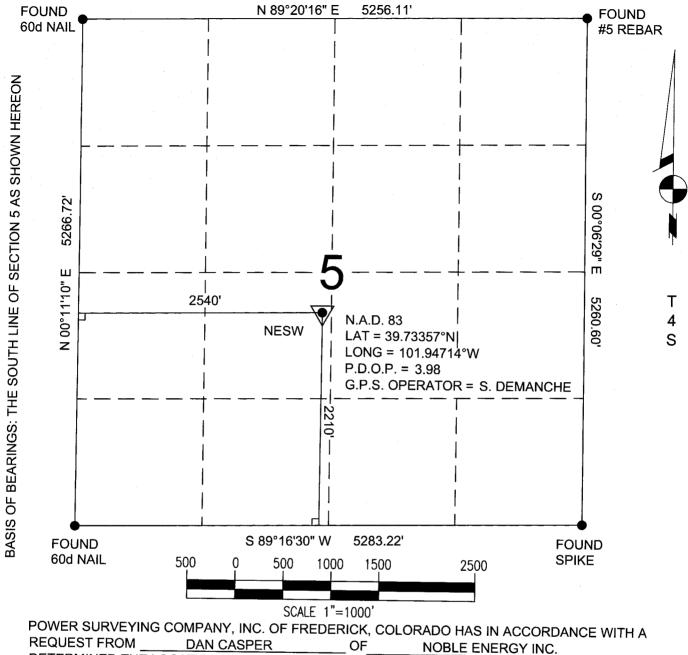
POWER SURVEYING COMPANY, INC. OF FREDERICK, COLORADO HAS IN ACCORDANCE WITH A REQUEST FROM \_\_\_\_\_ DAN CASPER OF \_\_\_\_ NOBLE ENERGY INC. \_\_\_\_\_ DETERMINED THE LOCATION OF \_\_\_\_\_ WIESE 23-5
