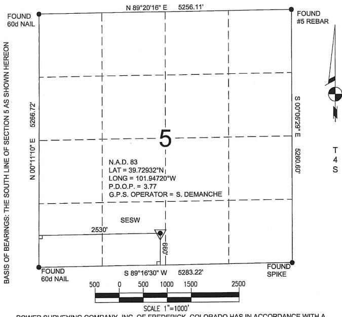
POWER SURVEYING COMPANY, INC. OF FREDERICK, COLORADO HAS IN ACCORDANCE WITH A NOBLE ENERGY INC. DAN CASPER REQUEST FROM **WIESE 24-5** DETERMINED THE LOCATION OF 660' FSL & 2530' FWL OF SECTION 5 TO BE OF THE PRINCIPAL MERIDIAN, , RANGE 41 WEST **TOWNSHIP** 4 SOUTH STATE OF KANSAS CHEYENNE COUNTY OF
