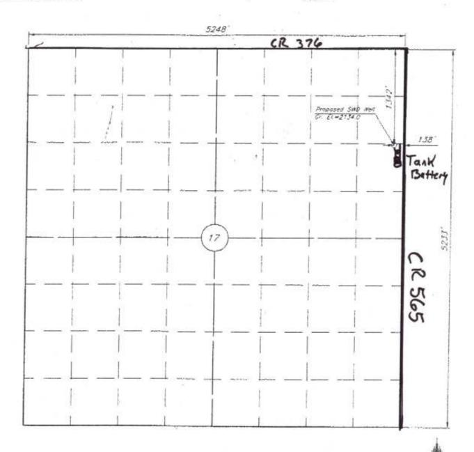
Elevations based on a Quad Map Elevation for the Northeast Corner of Section 17, 775, R21W. Elev. 2117.0
