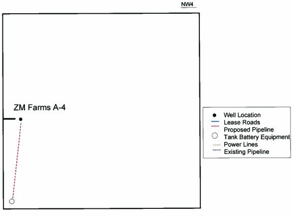
The PROPOSED Tank Battery for the ZM Farms A-4 will be located in the SW of the NW quarter.
