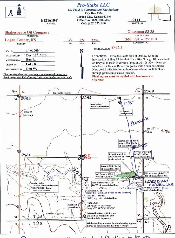
Preliminary non-binding estimate of flowlines, tanks, etc.
