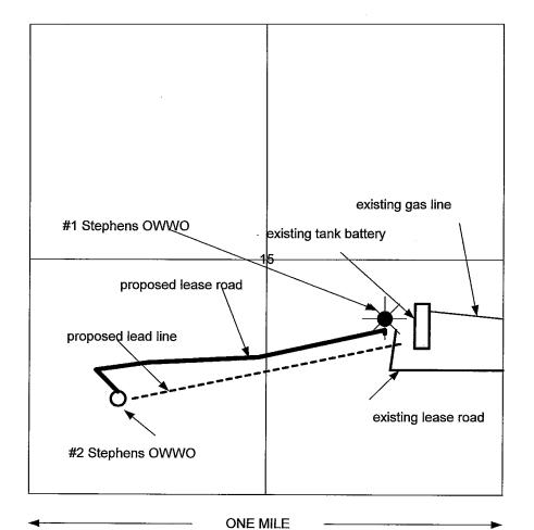
Plat showing proposed and existing roads, battery, and pipelines for the drilling and production of the #2 Stephens OWWO
