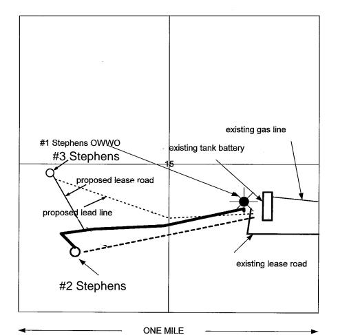
Plat showing proposed and existing roads, battery, and pipelines for the drilling and production of the #3 Stephens
