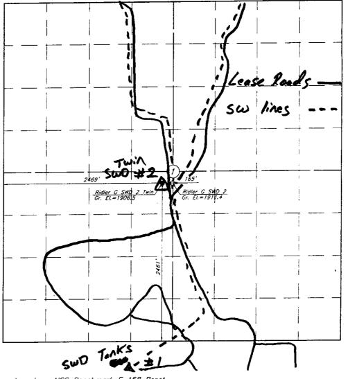
Elevations based on NGS Benchmark E 158 Reset. Standard disk located on the south end of the west hub guard of the Saline River bridge on U.S. Hwy. 183. NAVD 88 Sea Level Elevation= 1905.80 feet.
