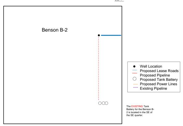
Proposed Details of SE/4 Sec 23 -T29S -R33W
