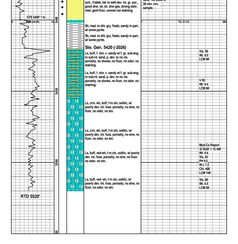
Attached to ACO-1 Form for WHITE EXPLORATION, INC. CARR #2-34 C E/2 SW/4 Section 34-29S-41W Stanton County, Kansas API# 15-187-21205-00-00
