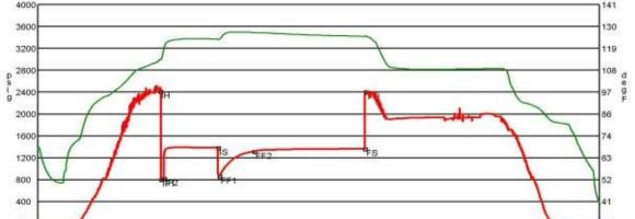
0 Time Pressure Temp 2/20/2012 1:14:10 PM 2/20/2012 1:16:00 PM 2/20/2012 1:20:30 PM 2/20/2012 2:50:30 PM 113.002 113.126 118.064 3.369444 2420.39 Initial Flow (1) Initial Flow (2) IF1 3.4 808.115 825.23 1383.305 3.475 4.975 IF2 IS Initial Shut-In 123.507 2/20/2012 2:50:30 PM 2/20/2012 2:52:40 PM 2/20/2012 3:50:50 PM 2/20/2012 6:54:50 PM 2/20/2012 6:57:10 PM Final Flow (1) Final Flow (2) 868.744 1316.459 123.391 5.011111
