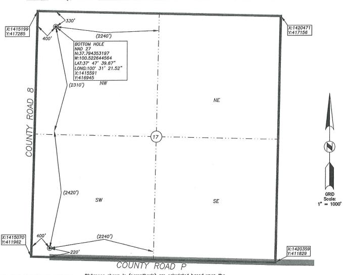
BOTTOM HOLE INFORMATION PROVIDED BY OPERATOR LISTED, NOT SURVEYED. CORNER COORDINATES ARE TAKEN FROM POINTS SURVEYED IN THE FIELD. Distances shown in (parenthesis) are calculated based upon the Quarter. Section being 2640 feet, those shown in [brackets] are based on GLO (General Land Office)distances and have NOT been measured on the ground.
