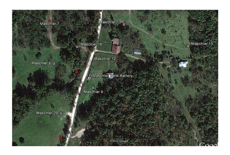
NEW INJECTORS ARE ON A 165 FOOT SPACING FROM EXISTING PRODUCERS
