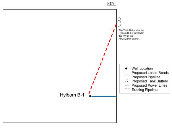
Proposed Details of NE/4 Sec 25 -T23S -R35W
