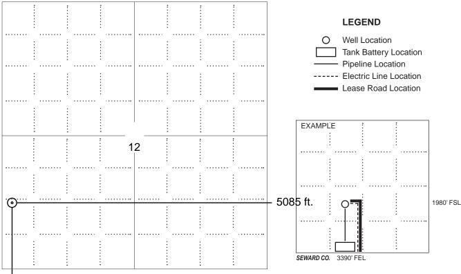
NQTE: In all cases locate the spot of the proposed drilling locaton.
