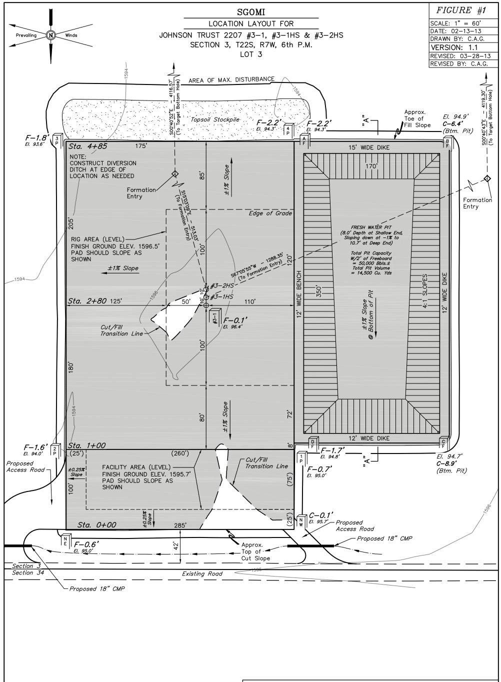
NOTE: Earthwork Calculations Require a Fill @ the Location Stakes For Balance. All Fill is to be Compacted to a Minimum of 95% of the Maximum Dry Density Obtained by AASHTO Method t-99.
