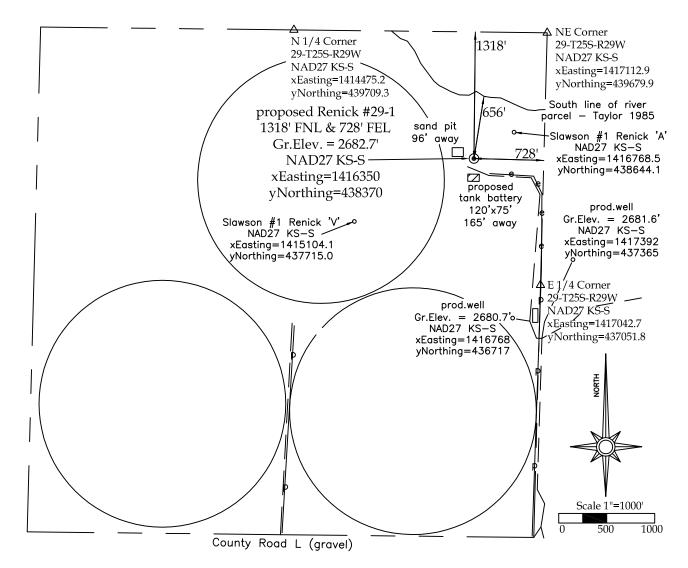
BASIS OF COORDINATES AND ELEVATION: NGS station Ingalls NAD83(1997) Lat 37 51 23.37640(N) Long 100 29 35.03091(W) and NAD27 KS-S N439271.9 E1424743.0 and Published Elevation 2795 feet.
