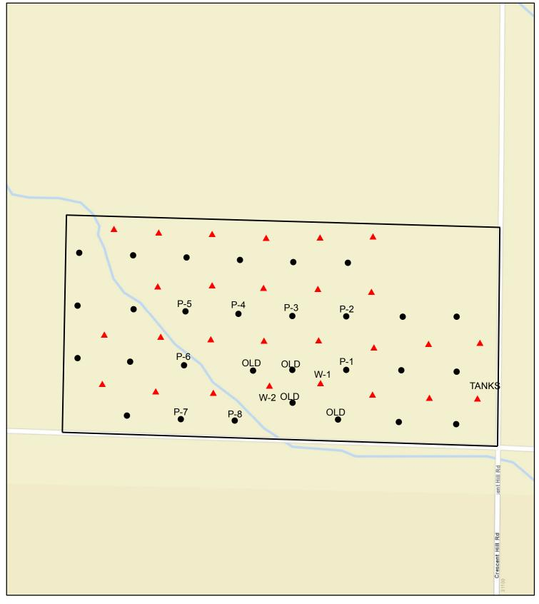
NEW PRODUCERS TO BE PLUMBED IN TO EXISTING WELL'S PRODUCTION AND ELECTRIC LINES
