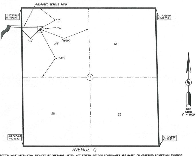
BOTTOM HOLE INFORMATION PROVIDED BY OPERATOR LISTED, NOT STAKED. SECTION COORDINATES ARE BASED ON OBSERVED POSSESSION EVIDENCE. DISTANCES SHOWN IN (PARENTHESIS) ARE CALCULATED BASED UPON THE QUARTER SECTION BEING 2640,00 FEET AND HAVE <u>NOT</u> BEEN MEASURED ON THE GROUND. PAD AND SERVICE ROAD LOCATIONS ARE SHOWN FOR GRAPHIC PURPOSES ONLY AND ARE NOT TO SCALE.
