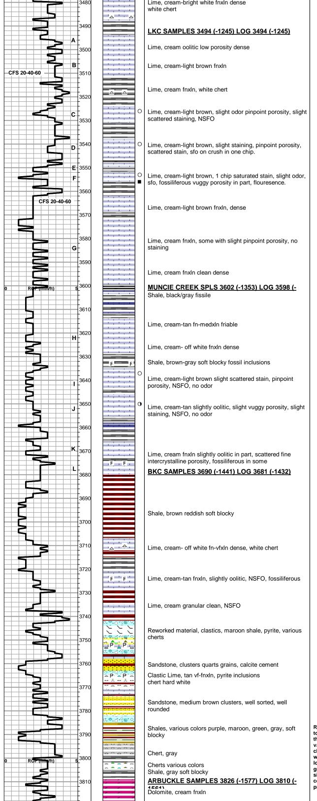
**Rock samples continued** to decline in quality throughout the well, various things were changed to correct this, with no success. Samples loaded with maroon and gray soft shale, carbonate sizes were very small. correlating samples proved to be very difficult.
