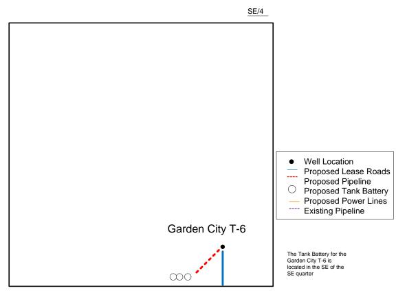
Proposed Details of SE/4 Sec 29-T23S -R34W
