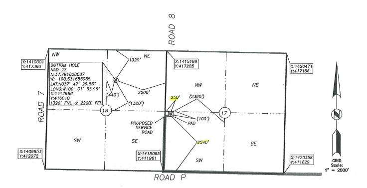
BOTTOM HOLE INFORMATION PROVIDED BY OPERATOR LISTED, NOT STAKED. SECTION COORDINATES ARE BASED ON OBSERVED POSSESSION EVIDENCE. DISTANCES SHOWN IN (PARENTHESIS) ARE CALCULATED BASED UPON THE QUARTER SECTION BEING 2640.00 FEET AND HAVE NOT BEEN MEASURED ON THE GROUND. PAD AND SERVICE ROAD LOCATIONS ARE SHOWN FOR GRAPHIC PURPOSES ONLY AND ARE NOT TO SCALE.
