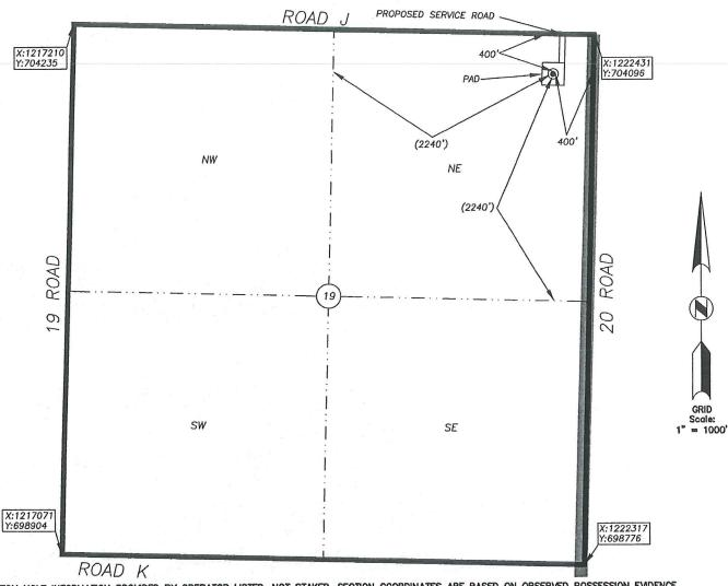
BOTTOM HOLE INFORMATION PROVIDED BY OPERATOR LISTED, NOT STAKED. SECTION COORDINATES ARE BASED ON OBSERVED POSSESSION EVIDENCE. DISTANCES SHOWN IN (PARENTHESIS) ARE CALCULATED BASED UPON THE QUARTER SECTION BEING 2640.00 FEET AND HAVE NOT BEEN MEASURED ON THE GROUND. PAD AND SERVICE ROAD LOCATIONS ARE SHOWN FOR GRAPHIC PURPOSES ONLY AND ARE NOT TO SCALE.
