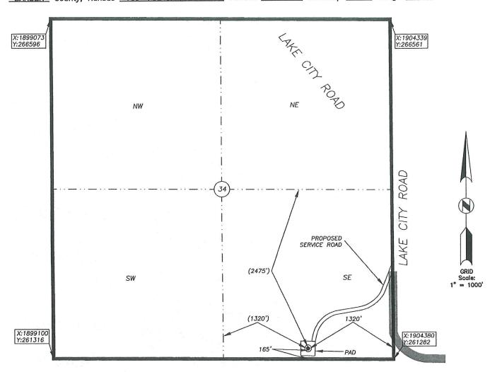
BOTTOM HOLE INFORMATION PROVIDED BY OPERATOR LISTED, NOT STAKED. SECTION COORDINATES ARE BASED ON OBSERVED POSSESSION EVIDENCE. DISTANCES SHOWN IN (PARENTHESIS) ARE CALCULATED BASED UPON THE QUARTER SECTION BEING 2640.00 FEET AND HAVE NOT BEEN MEASURED ON THE GROUND. PAD AND SERVICE ROAD LOCATIONS ARE SHOWN FOR GRAPHIC PURPOSES ONLY AND ARE NOT TO SCALE.
