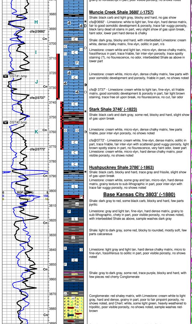
Mud-Co Mud Check -@3737 Wt: 9.25 Vis: 58 Pv: 15 YP; 18 pH: 10 WL: 9.6 -Cake 1/32nd Chl: 7,200 Cal: 0 Sol: 6.3 LCM: 0 -DMC: \$464.15 CMC: \$7,907.95 **Note Scale Change** C2 (units) C3 (uni Contaminated mud system Mud-Co Mud Check @3772 0810 hrs 12.11.13 Wt: 9.1 Vis: 49 Pv: 10 Yp: 23 pH: 9.0 WL: 14.2 Cake 1/32nd Chl: 12,800 Cal: 240 Sol: 5.0 LCM: Tr DMC: \$681.45 CMC: \$8,589.40 Total Gas (units
