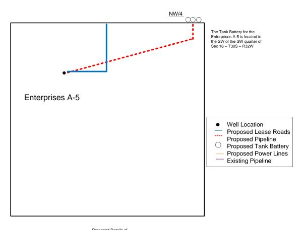
Proposed Details of SW/4 Sec 21 – T30S – R32W
