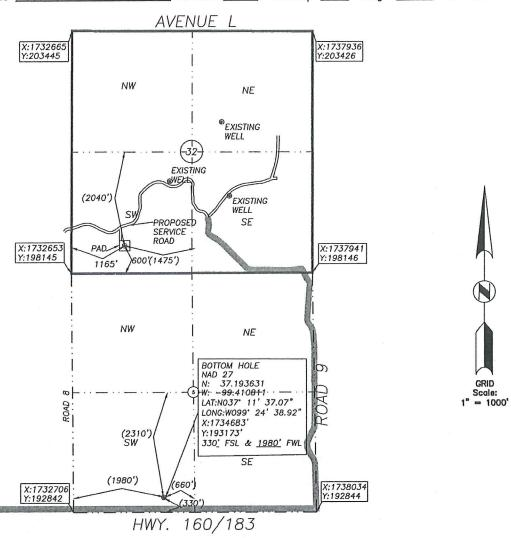
BOTTOM HOLE INFORMATION PROVIDED BY OPERATOR LISTED, NOT STAKED. SECTION COORDINATES ARE BASED ON OBSERVED POSSESSION EVIDENCE. DISTANCES SHOWN IN (PARENTHESIS) ARE CALCULATED BASED UPON THE QUARTER SECTION BEING 2640.00 FEET AND HAVE NOT BEEN MEASURED ON THE GROUND. PAD AND SERVICE ROAD LOCATIONS ARE SHOWN FOR GRAPHIC PURPOSES ONLY AND ARE NOT TO SCALE.
