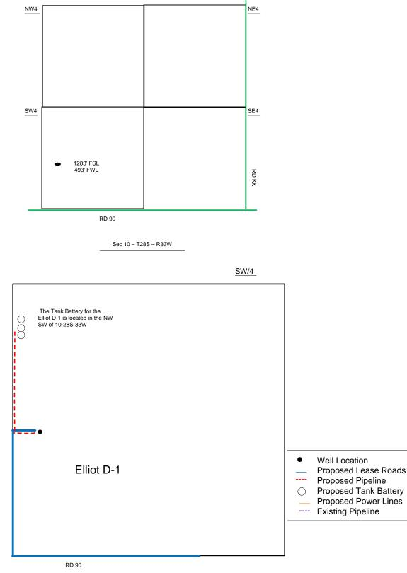
Proposed Details of SW/4 Sec 10 - T28S - R33W
