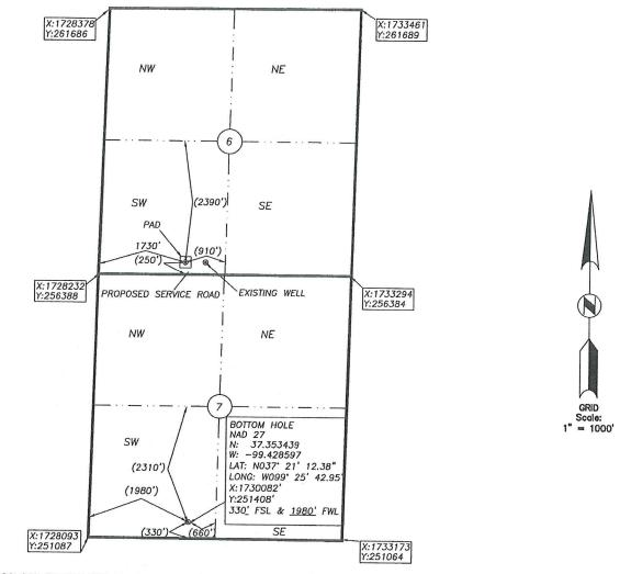
BOTTOM HOLE INFORMATION PROVIDED BY OPERATOR LISTED, NOT STAKED. SECTION COORDINATES ARE BASED ON OBSERVED POSSESSION EVIDENCE. DISTANCES SHOWN IN (PARENTHESIS) ARE CALCULATED BASED UPON THE QUARTER SECTION BEING 2640.00 FEET AND HAVE NOT BEEN MEASURED ON THE GROUND. PAD AND SERVICE ROAD LOCATIONS ARE SHOWN FOR GRAPHIC PURPOSES ONLY AND ARE NOT TO SCALE, SANDRIDGE EXPLORATION AND PRODUCTION, LLC, **OPERATOR:** LEASE NAME: FI FVATION. MURPHY 3119 WELL NO: 3-7H
