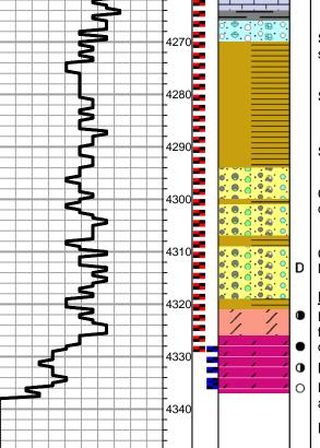
Shale, grayish green grading into vari colored shales, slightly waxy
