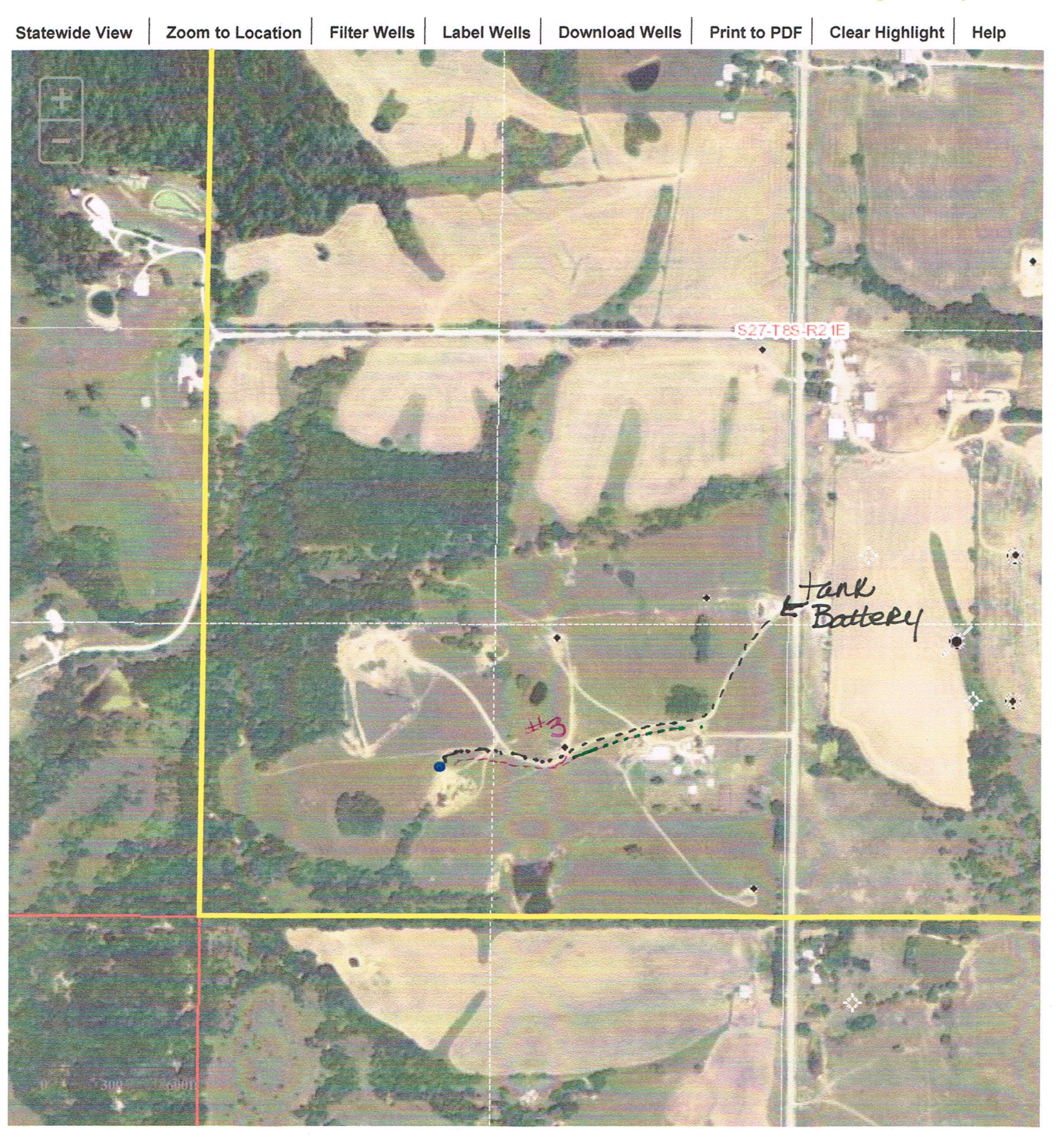
Well#6 in Blue tank Battery shown Right Middle. Roads Shown to well to outlined in Black-dotted line Ditch w/ pipeline & Stectrical will be burried south of Road-dotted line, will tie in at Well#3
