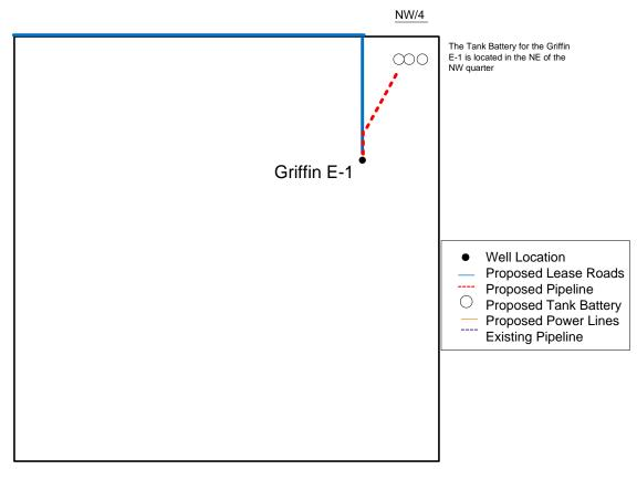
Proposed Details of NW/4 Sec 11 – T28S – R33W
