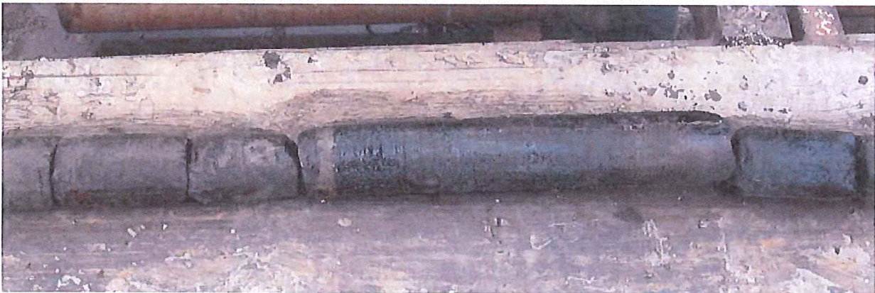
Middle Squirrel Sandstone, 1338' to 1341', Unrinsed Core
