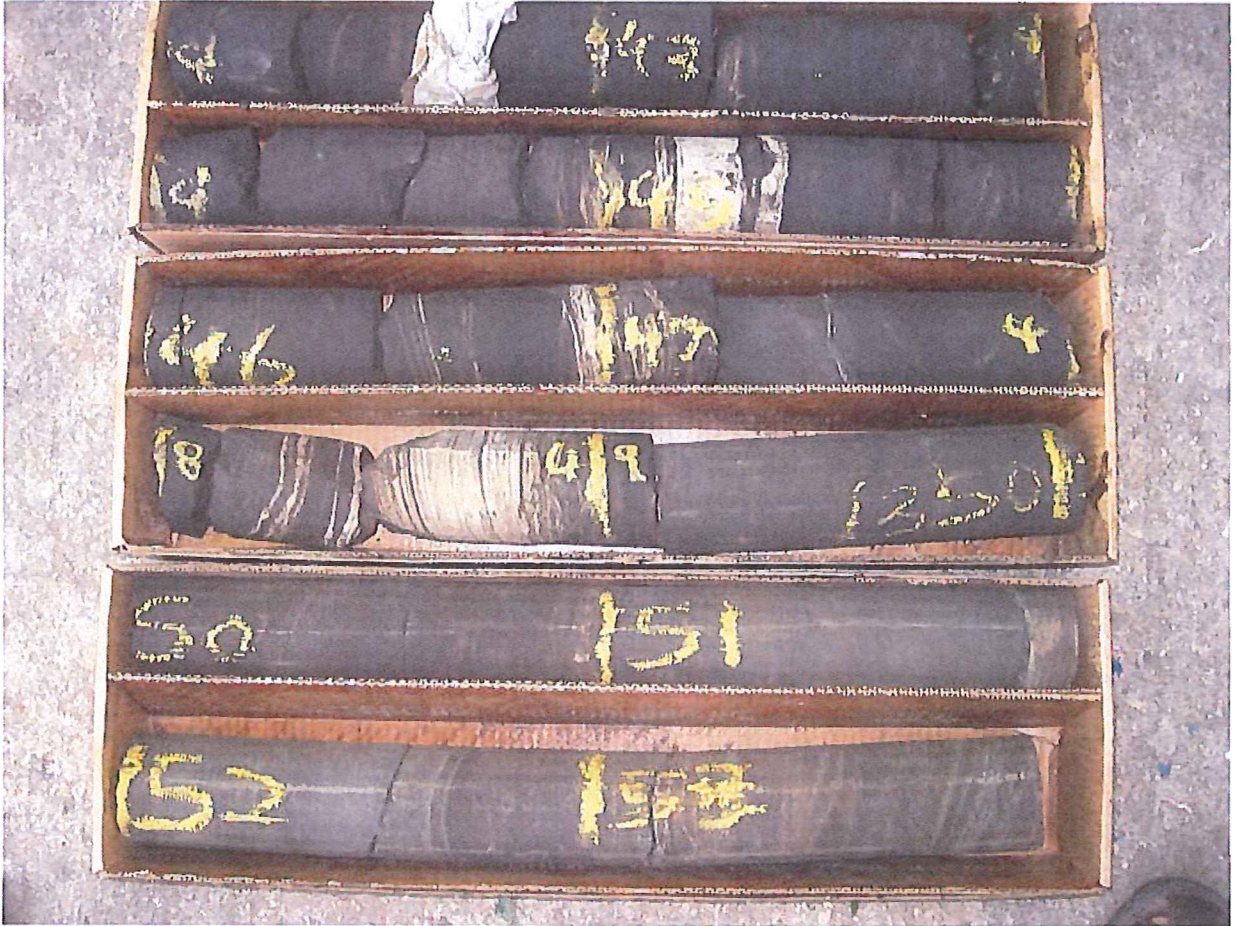
Middle Squirrel Sandstone, 1342' to 1354', Dry Core
