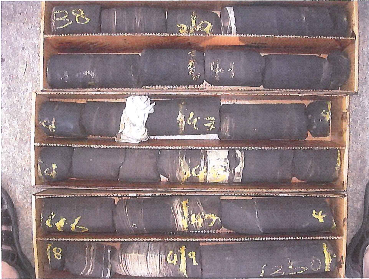
Middle Squirrel Sandstone, 1338' to 1350', Dry Core
