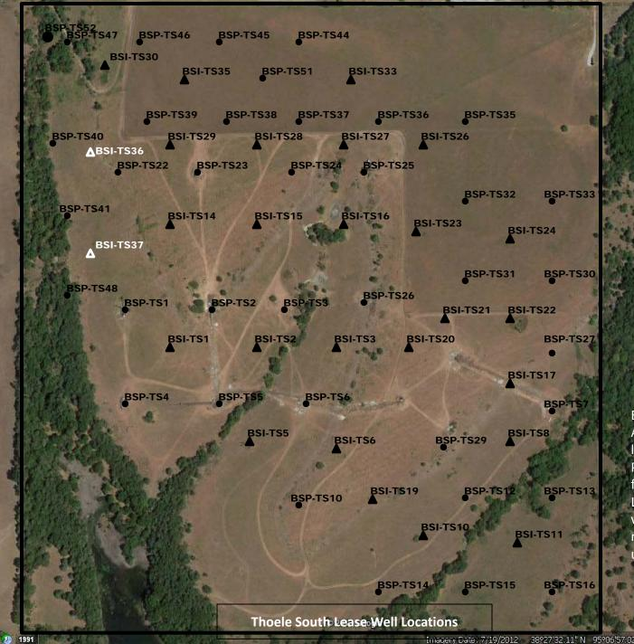
Electrical and tanks Are located on adjoining lease to the South. Pipelines and flow lines follow the lease roads. Lease roads where not visible on aerial map, the most direct route in used.
