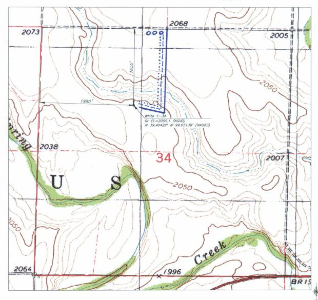
Elevations based on a USGS Quad Map Elevation tied to the Northwest Corner of Section 34, T7S, R21W. Elev.=2073.00
