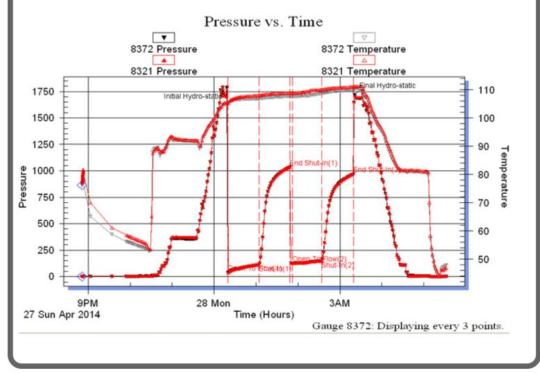
Well Name & No.: Sack #1 Company: Hess Oil Company Test No.: 5 Interval Tested: 3698 - 3710 Zone Tested: Marmaton Times: Miss Run (Packer Failure) Blow Description: IFP: ISI: FFP: FSI: Rec: 200 Feet of M, 1000% Mud Rec. Total: 200°, BHT: N/C Gravity: N/C
