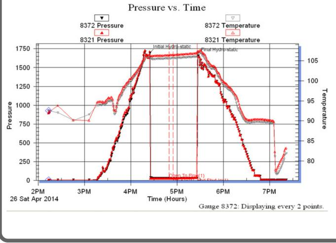
Well Name & No.: Sack #1 Company: Hess Oil Company Test No.: 3 Interval Tested: 3474-3520
