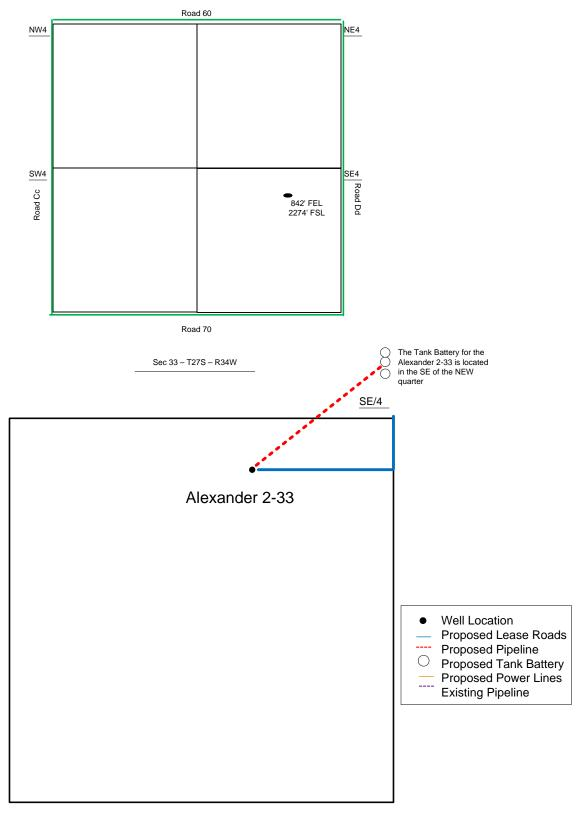
Proposed Details of SE/4 Sec 33 – T27S – R34W
