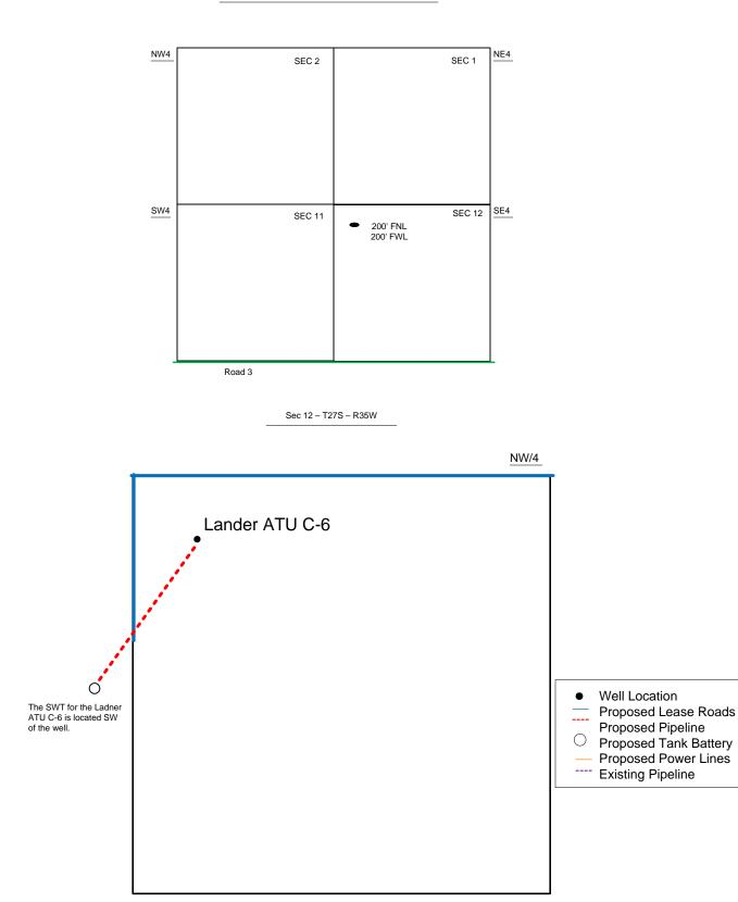
Proposed Details of NW/4 Sec 12 – T27S – R36W Proposed Site Diagram Ladner ATU C-6 August 5, 2014
