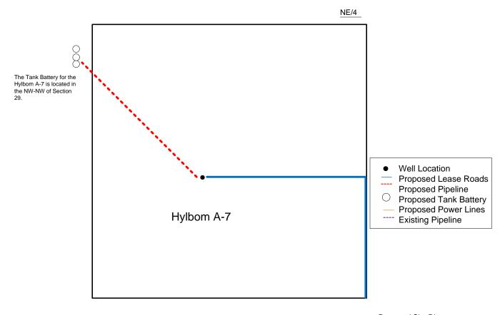
Proposed Details of NE/4 Sec 30 – T23S – R34W Proposed Site Diagram Hylbom A-7 August 19, 2014
