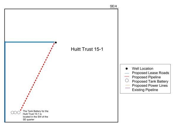
Proposed Details of SE/4 Sec 15 – T30S – R33W
