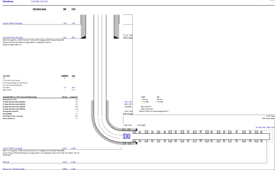
11.6# N-80: Cplg OD =5.000" ID=4.000" Drift=3.875" Collapse= 6350 Internal Yield=7780
