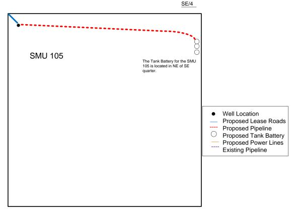
Proposed Details of SE/4 Sec 28 – T23S – R34W
