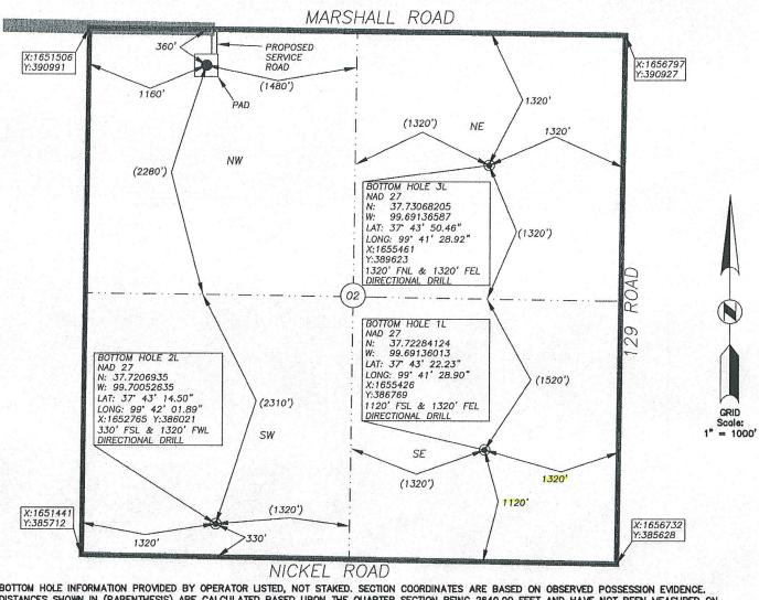
BOTTOM HOLE INFORMATION PROVIDED BY OPERATOR LISTED, NOT STAKED. SECTION COORDINATES ARE BASED ON OBSERVED POSSESSION EVIDENCE. DISTANCES SHOWN IN (PARENTHESIS) ARE CALCULATED BASED UPON THE QUARTER SECTION BEING 2840,00 FEET AND HAVE <u>NOT</u> BEEN MEASURED ON THE GROUND. PAD AND SERVICE ROAD LOCATIONS ARE SHOWN FOR GRAPHIC PURPOSES ONLY AND ARE NOT TO SCALE,
