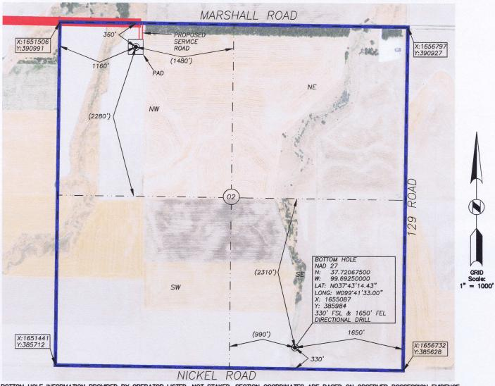
BOTTOM HOLE INFORMATION PROVIDED BY OPERATOR LISTED, NOT STAKED. SECTION COORDINATES ARE BASED ON OBSERVED POSSESSION EVIDENCE. DISTANCES SHOWN IN (PARENTHESIS) ARE CALCULATED BASED UPON THE QUARTER SECTION BEING 2640.00 FEET AND HAVE NOT BEEN MEASURED ON THE GROUND. PAD AND SERVICE ROAD LOCATIONS ARE SHOWN FOR GRAPHIC PURPOSES ONLY AND ARE NOT TO SCALE.
