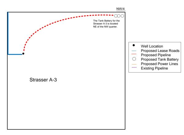
Proposed Details of NW/4 Sec 28 – T23S – R32W
